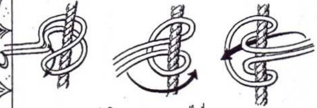
Prusik Best friction knot for rope ascent without jumars. Loop a sling of 5-7 mm rope around top rope and feed it back through itself 2 or 3 times.
